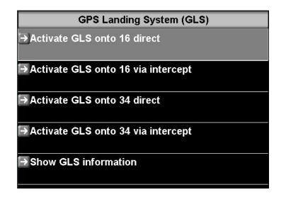
You can activate a GLS approach either direct (the HSI will be set to ILS mode) or you can first navigate to an intercept point along the extended runway centerline (the distance from the touch down point is set in the GVOR/GLS setup menu, for example 5Nm).
