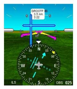
Textual information shows that we are 3.5 nm from GROOTF and need 3 minutes, 22 seconds to touch down at current speed. The HSI shows we are to the right of the runway.
