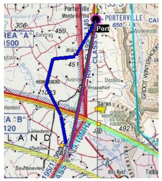
Simply tap on the map to outline the divert you want to fly. Here we tapped on 4 locations to the left of our track. The divert is not yet active and is shown in blue. We can at this stage press "cancel" to return to normal mode (and forget the divert), we can remove the last point defined (if we made a mistake or want to change the location a bit) and if we are happy with our divert we can activate it:
