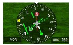
VOR NAV is described in mode detail further down in this document. The system provides for a primary and secondary VOR source showing "paddles" that give you an indication where these sources are located (from a direction point of view). The radials from these VOR stations are shown as lines.
