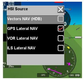
Selecting a GPS waypoint, activating a route (flightplan), selecting GVOR primary or activating a GLS selects the navigation source automatically.
