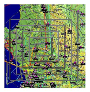
The box starts slightly offset to the right in this case to give even coverage. The lanes are 4NM apart giving us 2NM to each side minimum observability.
