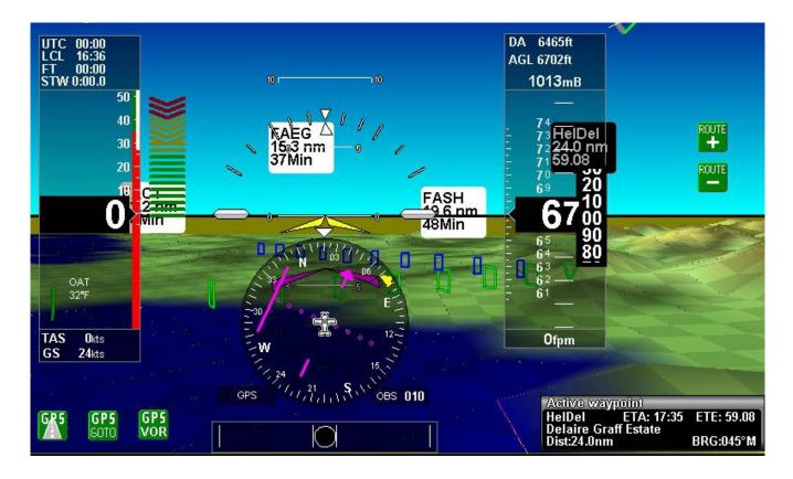
Typical screen display with a route active. Note the Route+ and Route- buttons. Also note the highway in the sky presentation to the next waypoint shown with a green triangle. The green highway is your current track and you are within 180 degrees of ground track to this track. If you are more than 180 degrees deviant, the green highway turns to a red highway.
