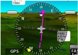
This is also the only NAV source the system will automatically select in some cases. For example, regardless of currently selected NAV source, if you perform a "direct-to" waypoint selection the NAV source will be immediately selected to GPS Lateral NAV for you to reduce your workload.
