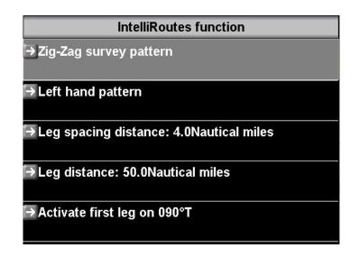
The "Zig-Zag" survey pattern creates a "back and forth" pattern of a defined leg distance and lane spacing. The left or right hand pattern defines the direction of the first turn.
