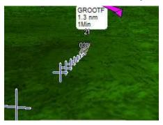
This image shows approach guidance onto runway 03 at GROOTF. Approach guidance is shown with blue crosses on a white background. The glide slope angle is based on the angle selected in your GLS setup (typically 3.0 degrees).
