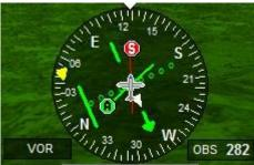
HSI showing both primary and secondary GVOR stations. The red (S) paddle shows the direction of the location of the secondary VOR station.
