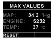
This display can be accessed by rotating the rotary control during the normal display mode. Press the F1/Up button when the max values display is showing to reset the maximum values to the current values.
