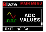
This menu displays the ADC values that have been read from the pressure and temperature sensor.
