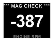
Press the F2/Down button once you have reached your normal run-up RPM. The display will show the RPM deviation from when the magneto function was activated. Any RPM drops will be displayed as a negative RPM value, a positive reading indicates an increase in RPM.
