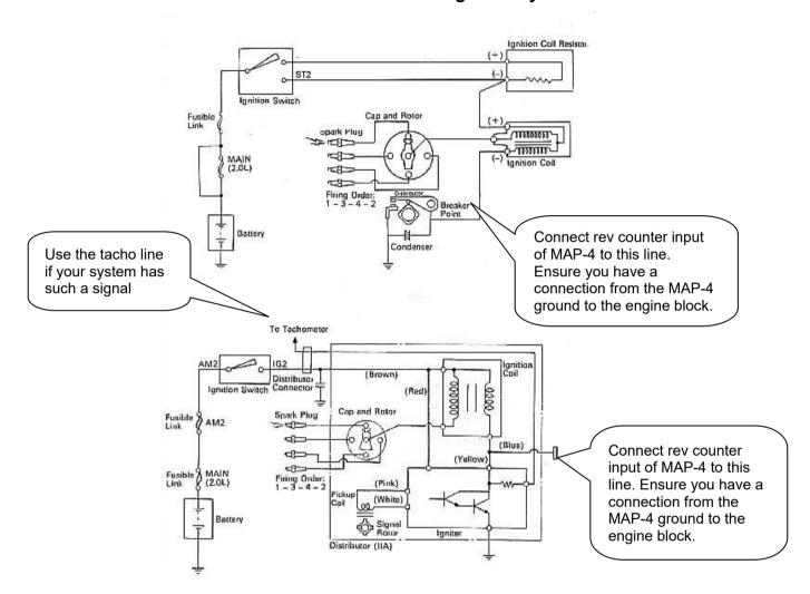
Electronic ignition system with conventional ignition coil
