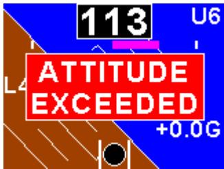
Message displayed when the maximum bank, pitch or yaw rates have been exceeded
